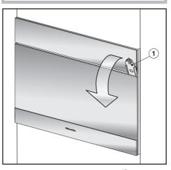
Insert the opener supplied ① about 3 cm into the gap between the door and the control panel on the right hand side and then pull the door open.
